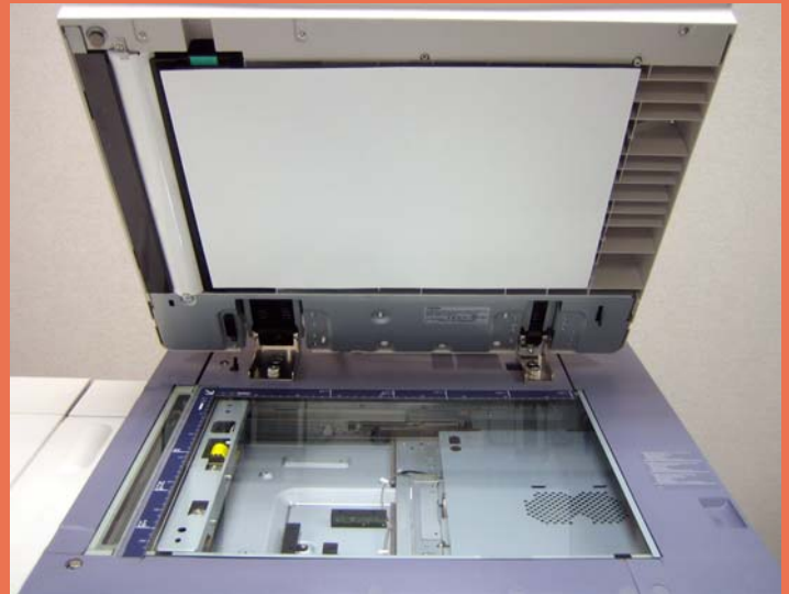
Above and below: The E-Studio 4520C's platen (above) and document feeder (below), with the document feeder's cover opened in order to expose the feeder's misfeed-access area.
