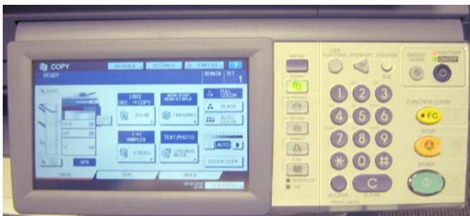
The E-Studio 4520C's Control Panel consists of a touch screen and hard keys.
