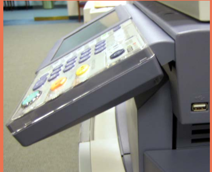
The Control Panel can be tilted in order to eliminate any glare, as well as to make it easier for wheelchair users to view and operate.
