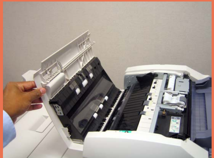
Above and below: The E-Studio 4520C's platen (above) and document feeder (below), with the document feeder's cover opened in order to expose the feeder's misfeed-access area.
