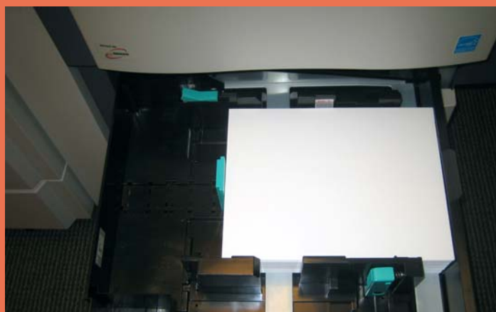
Both tray 1 and tray 2 can each hold 550 sheets of 20 lb. Bond /80 gsm or 500 sheets (105 gsm or 28 lbs bond media (in from 5.5"x8.5"/A5-R up to 11"x17"/A3).
