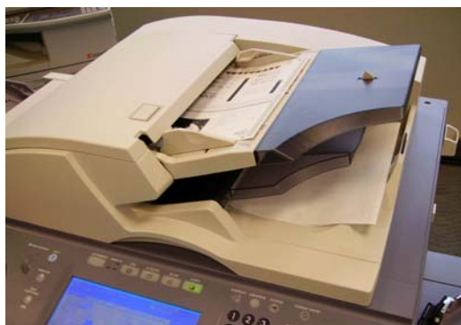
The automatic document feeder of the e-STUDIO600 is convenient to use—and fast, scanning up to 71 ppm at 600 dpi resolution.
