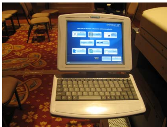
Above: ScanStation touchscreen interface Below: Swivel-mounted stand
