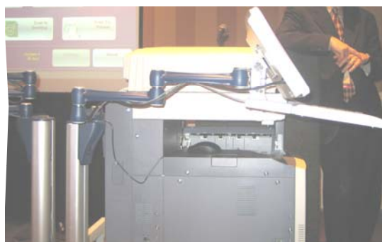
Above: ScanStation touchscreen interface Below: Swivel-mounted stand
