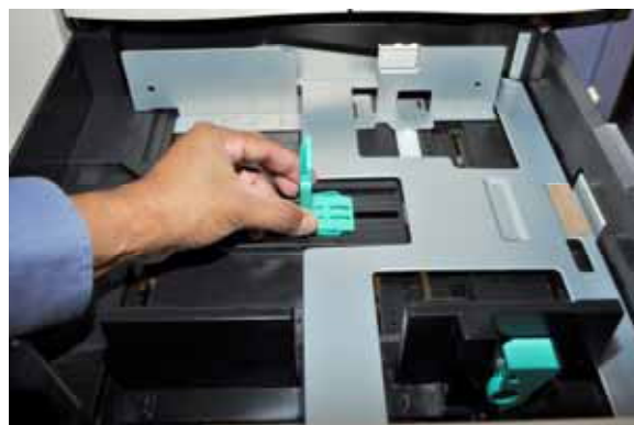
Above and next column: In order to adjust the paper cassettes to accommodate different paper sizes, the user squeezes and slides these green guides into place. BERTL found it easy to adjust the paper cassettes.
