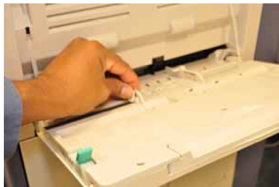
The 100-sheet bypass tray can be adjusted by sliding these levers into place. The feeder can be adjusted for envelope and tab printing.
