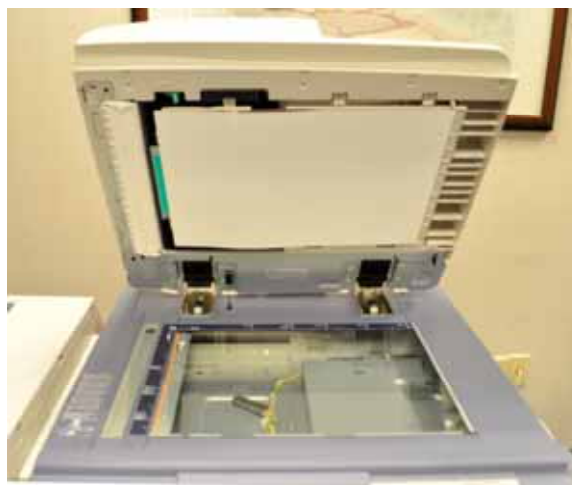
Above and next page: The Toshiba e-STUDIO855 platen glass and automatic document feeder (ADF).
